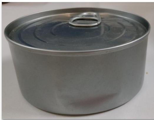
Fig. 1. Abolladura Leve (Grado 2)
