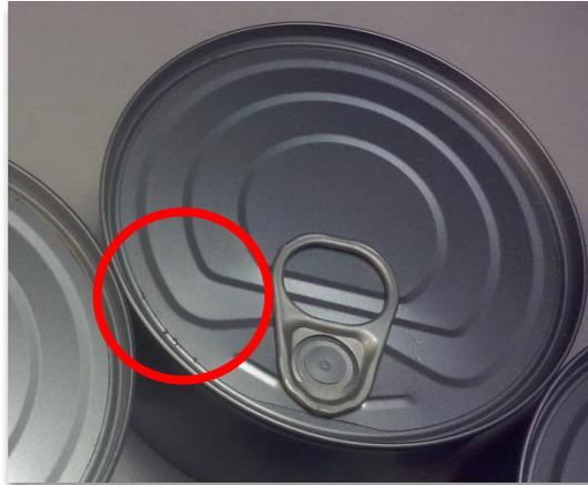
Fig. 4. Oxido Leve (Grado 2)
