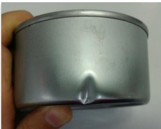
Fig. 2. Abolladura Leve (Grado 2)
