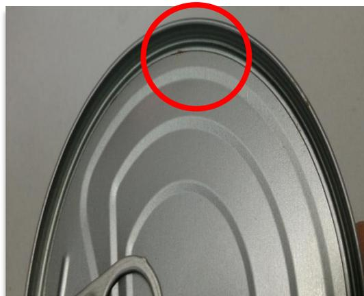
Fig. 5. Oxido Leve (Grado 2)
